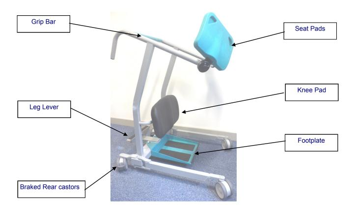
The seat pads can swivel as shown in the photograph opposite. This allows the transfer aid to get as close as possible to the client. Position the transfer aid and apply the rear castor brakes, so the client can step onto the foot plate. Ensure that the client has hold of the grip bar, before rotating the seat pads back to the operating position.
